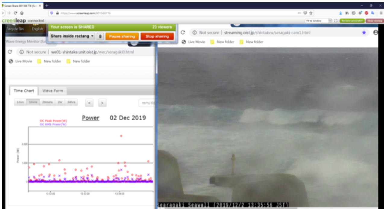
Figure 3. OIST-Wave Energy Converter monitoring screen. A CCTV camera is installed on the Seragaki's seawall facing the device and the power generated data is uploaded to data storage at OIST via cloud storage.
