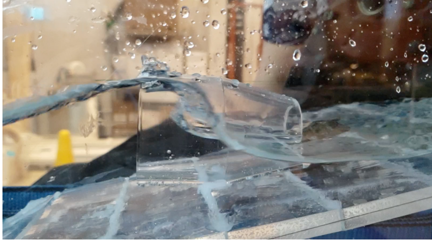
Figure 1. Small scale (1:20) physical model of the Taper-Duct experiments using the small wave flume at OIST against regular breaking wave. A motorised wave paddle is utilised to generate the breaking wave.
