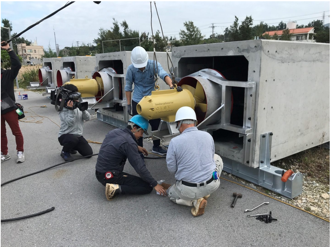
Figure 4. Four (4) Taper-Ducted OIST Wave Energy Converter devices being prepared at the Port of Seragaki before being sent to Kandooma Beach, Maldives, by ship.
