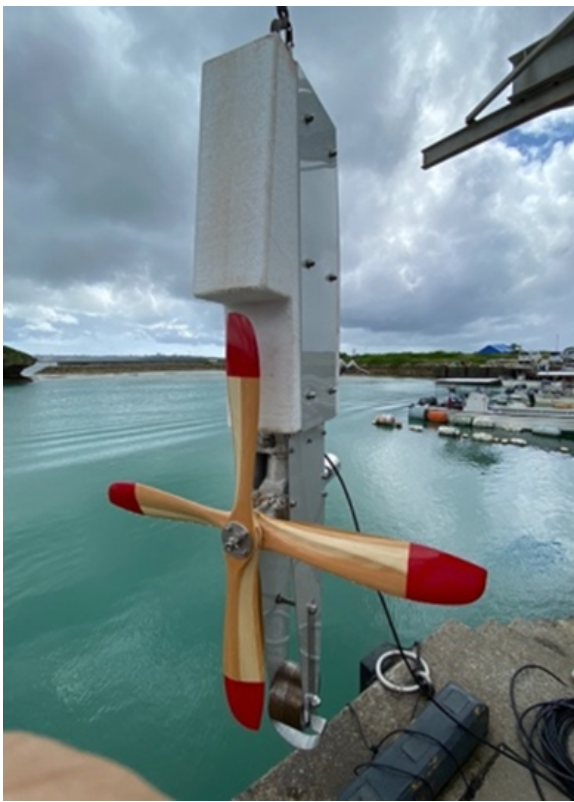
Figure 4. The first demonstration model using half-scale generator with propellers from the powered paragliders. The turbine is located behind of the float, and thus this design is "down wind" type, which causes the shadow problem on the turbine, i.e., lowering the speed of water.
