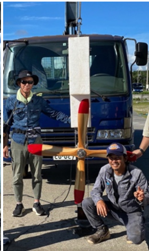
Figure 4. The first demonstration model using half-scale generator with propellers from the powered paragliders. The turbine is located behind of the float, and thus this design is "down wind" type, which causes the shadow problem on the turbine, i.e., lowering the speed of water.
