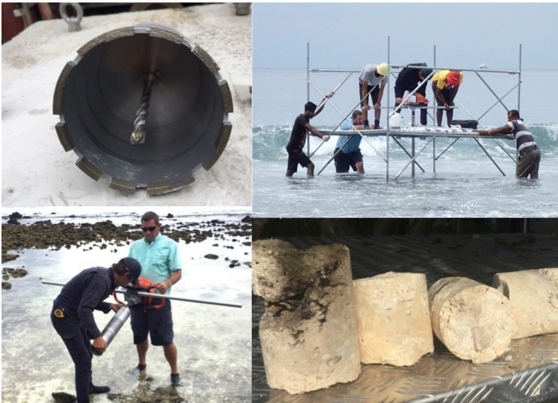
Fig. 4. Drilling into the sea floor with core drill. We used a gasoline engine (75 cc cylinder two-cycle) to drive the core drill.
