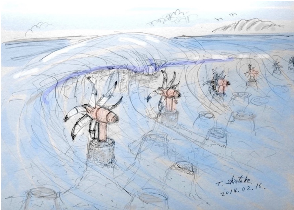
Fig. 1. Arrays of small turbines harness electricity from the rapid flow of breaking waves on shore. They would act as a wave breaker to damp the wave by extracting its kinetic energy.
