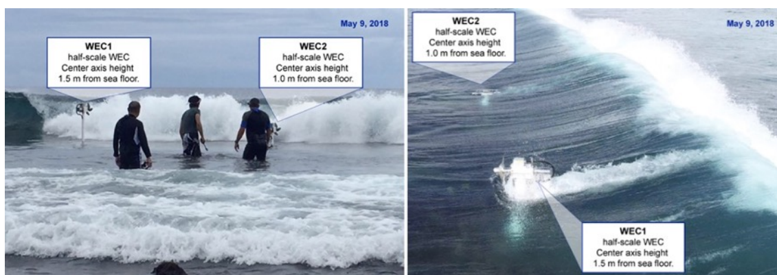
Fig. 8. (left) Strong surf wave breaks in front of WECs, (right) two WECs standing and generating electricity daily in the breaking waves.
