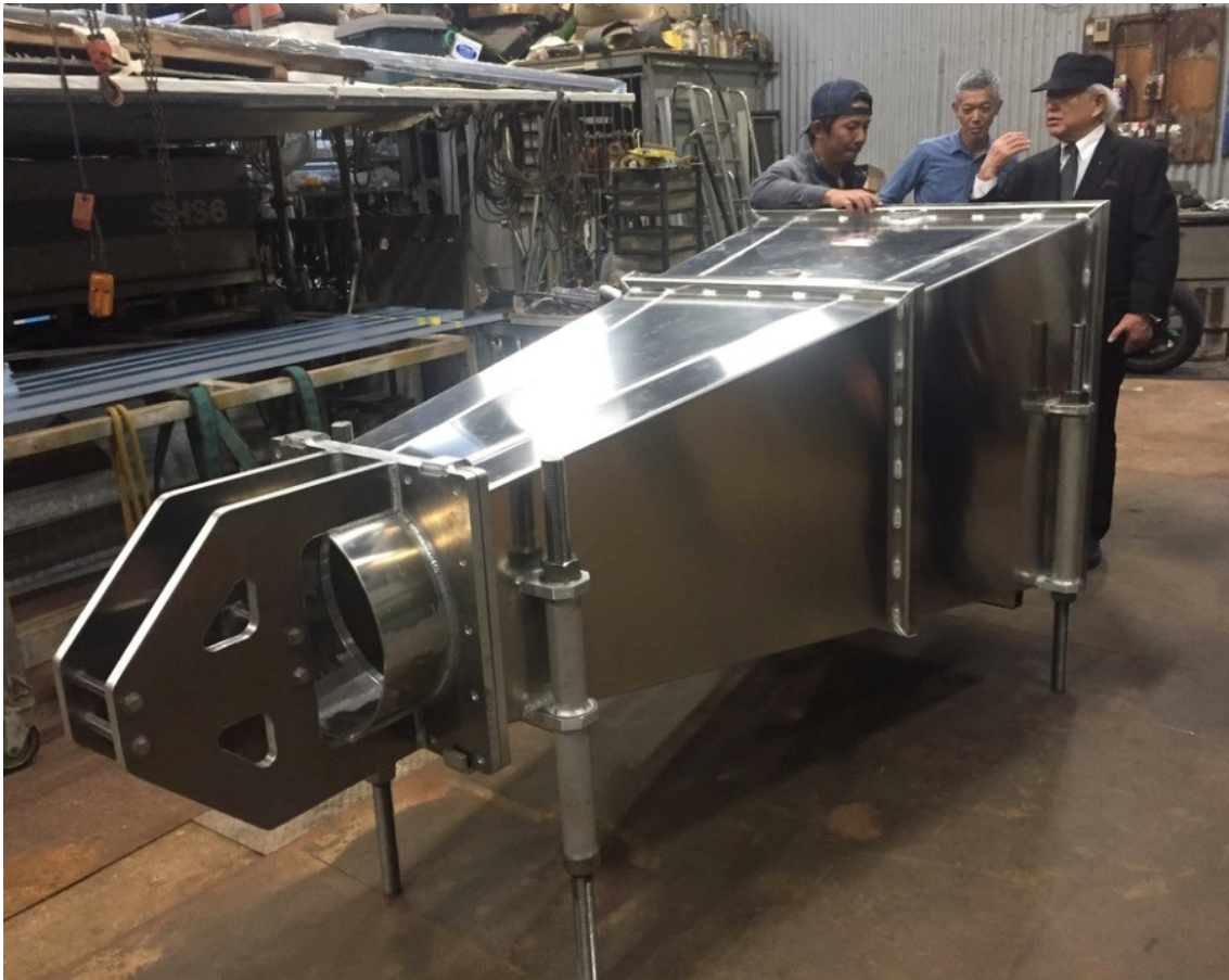
Fig. 19. Ducted-WEC concept, and 1st prototype model made by aluminum plate. We attached the half scale WEC to the end of this taper.
