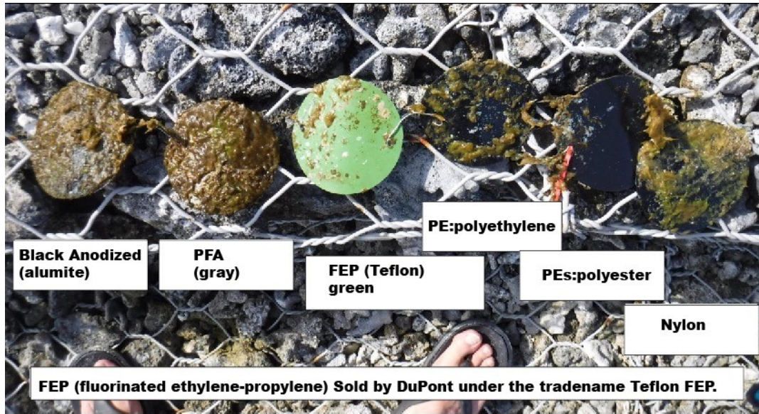
Fig. 16. Two and half months seawater test in Maldives. FEP(Teflon) and PEs Polyester are suitable to reduce algae growth
