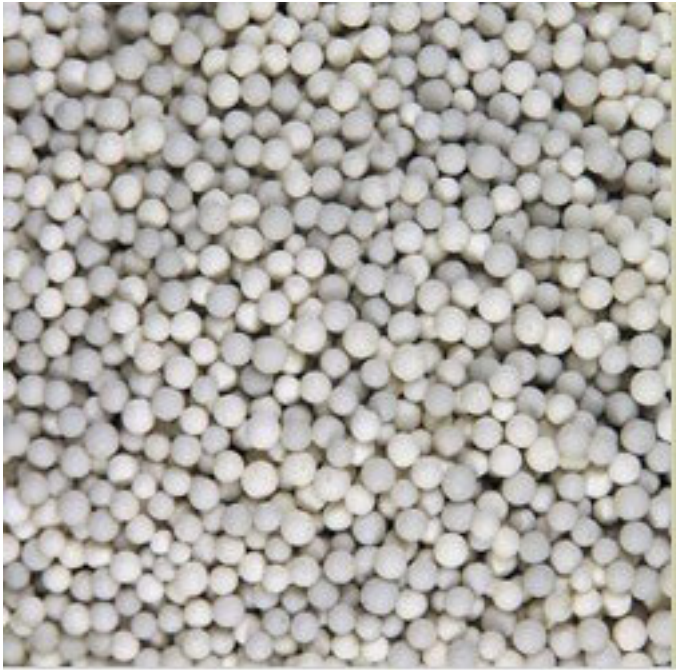
Fig. 6. We filled the ceramic balls (porcelain) of 2~3 mm diameter in the cylindrical gap, to form a crystal-like rigid structure and support the socket. The repeating vibration by the breaking wave improves the filling factor inside the packed balls with self-aligning mechanism.
