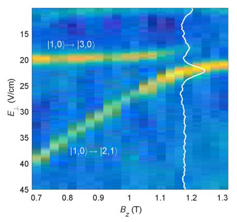
In our experiments, we create this situation by applying a *B*-field which is tilted with respect to the surface of liquid helium and performing the Stark spectroscopy of electron's energy levels. We find a variety of phenomena reminiscent of those studied in Atomic and Molecular Optics (AMO), such as sideband transitions, avoid crossings, Lamb shift, etc. We are interested in exploiting the non-linearity introduced by this coupling and performing cQED experiments with this system.
