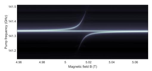
In our experiments, we realize the strong coupling between an ensemble of 2D electrons on helium and a single-mode Fabry-Perot cavity resonator working in a millimeterwave frequency range. We are interested in the study of non-linearities in this coupled system and their potential use for creation of non-classical states of light and matter.
