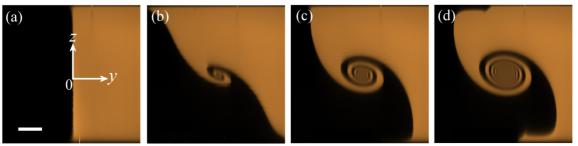
Development of the spiral vortex structure in the x = 0 plane as the Reynolds number (Re) is varied: (a) Re = 15.2, (b) Re = 42.8, (c) Re = 60.6, (d) Re = 91.0. Scale bar in (a) represents 200  $\mu$ m.
